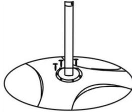
Fix the bottom tube to the base by using 4 pcs 6\*35 mm screws.
