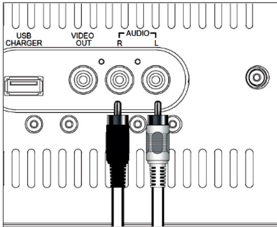
Connect an RCA video cable to the RCA Video Output on the karaoke machine and a video input on a television. Adjust the television source to the input used:
