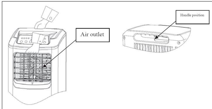
**Note:** Do not hold the horizontal louvre by hand. Leave the unit in the upright position when handling or moving it. If the remote control is in the position of the handle, take out the remote control.
